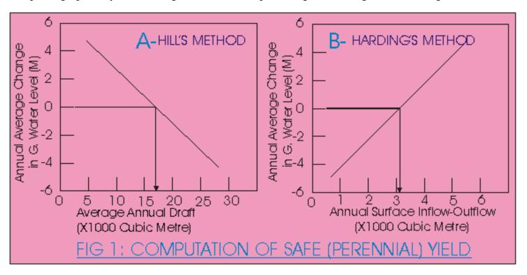
ground water level. If the water supply to the basins is reasonably constant a straight line can fit the points. The draft corresponding to zero change in the elevation equals the safe yield. The method has the advantage that the draft during the entire period of record may be an overdraft, yet the prolongation of the fitted straight line defines the safe yield at the intercept of the zero change in elevation line (figure 1A).
