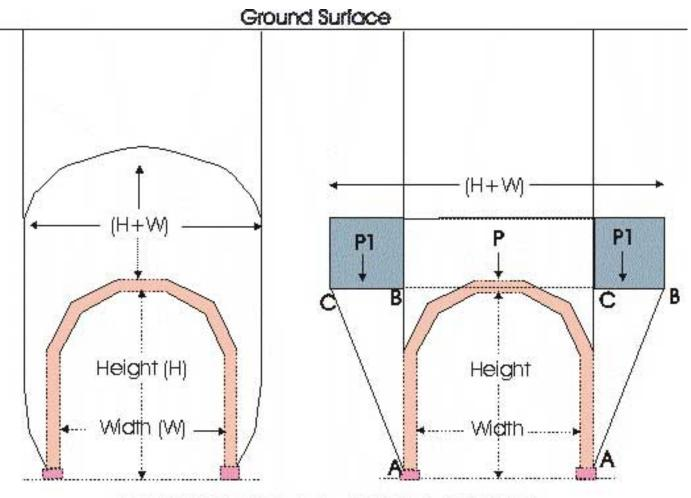
PRESSURE ON A TUNNEL LINING
